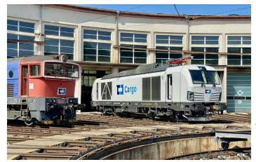
Operation of the locomotive is possible on non-electrified lines and lines with a 15kV/16.7 Hz supply system. That's why it makes it possible to effectively serve non-electrified private sidings or loading yards and then, without any redundant locomotive swapping and time delays to carry the goods as far as to the destination on electrified lines. German branch of ČD Cargo deploys this locomotive for instance on scrap iron trains or trains carrying chemical products.
