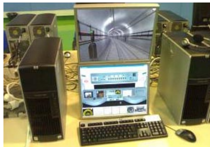
Figure 32: Example of a simulator with software interface of cab equipment at Metro de Madrid, Spain
